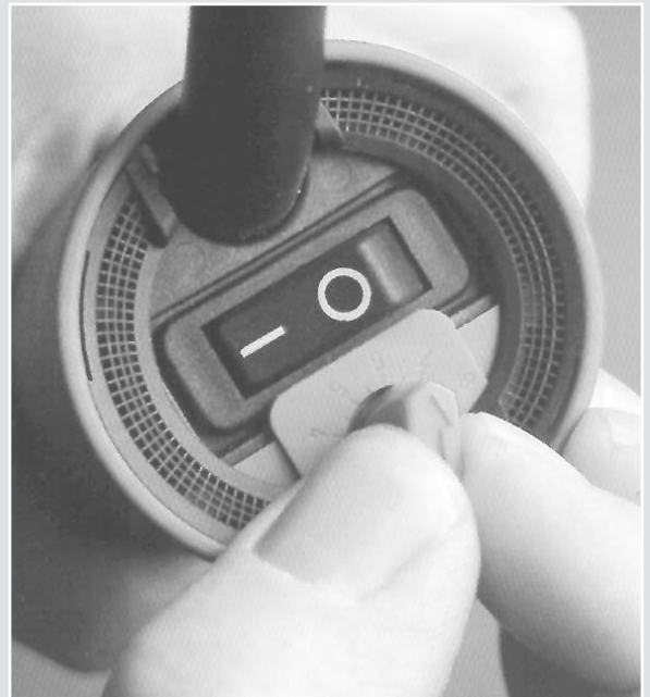
The rotary control on the rear of the hot-air tool enables accurate setting of welding temperatures up to 700°C.
